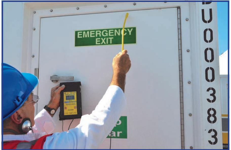
**DOOR-SAFE™** is an American Bureau of Shipping (ABS) Type Approved ultrasonic unit that provides a quick and simple method of establishing water and weather tightness in doors, hatches and windows.
