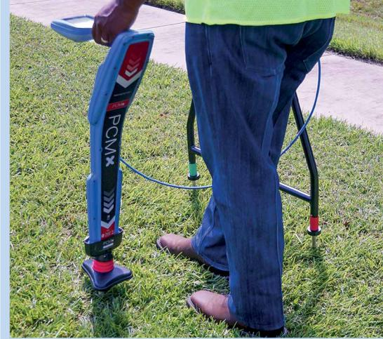
One second mapping measurements combined with simultaneous ACCA and ACVG data gathering makes surveying faster.
