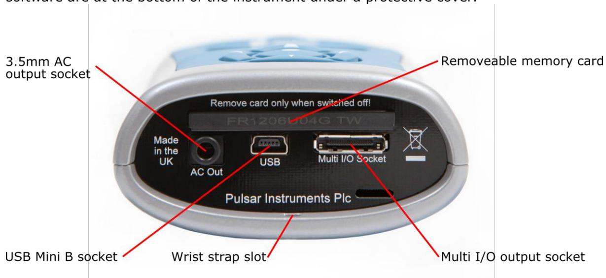
The Nova® can be powered via the multi-pin connector on the bottom of the instrument.
