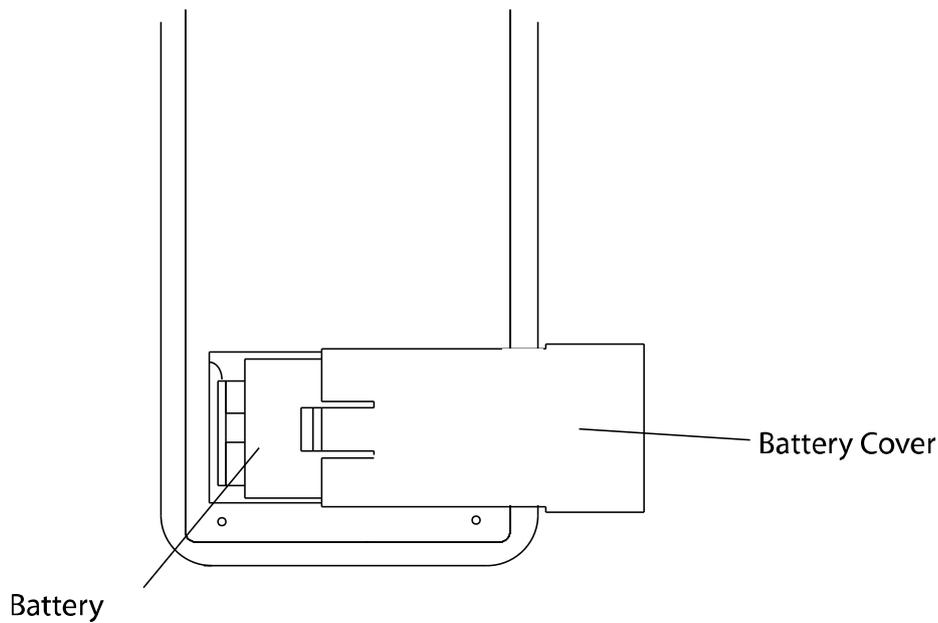
1. Ensure the instrument is turned off before removing the battery cover.
