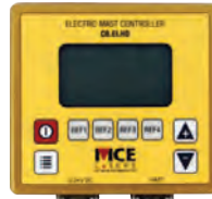
CB.EI.HD - elevation indicator for use with ME.14 electric mast. Features 4 memory settings for easy storing and recalling of 4 different height values. Mast will automatically adjust to the stored height values when selected at the press of a button.
