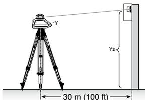
6. After checking the Y-axis, rotate the laser 90°. Repeat the above starting with the + X axis facing the wall.
