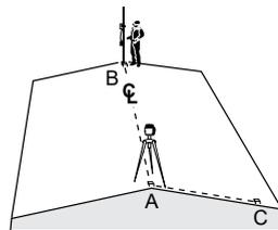
6. Set the grade rod on the slope axis direction hub to adjust the laser's elevation without changing the height of the receiver on the grade rod (C).
