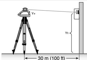
3. Rotate the laser 180° (-Y axis toward the wall) and allow the laser to re-level.
