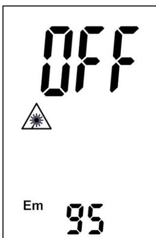
"Off" or "On" indicates whether the laser pointer is switched off or switched on.
