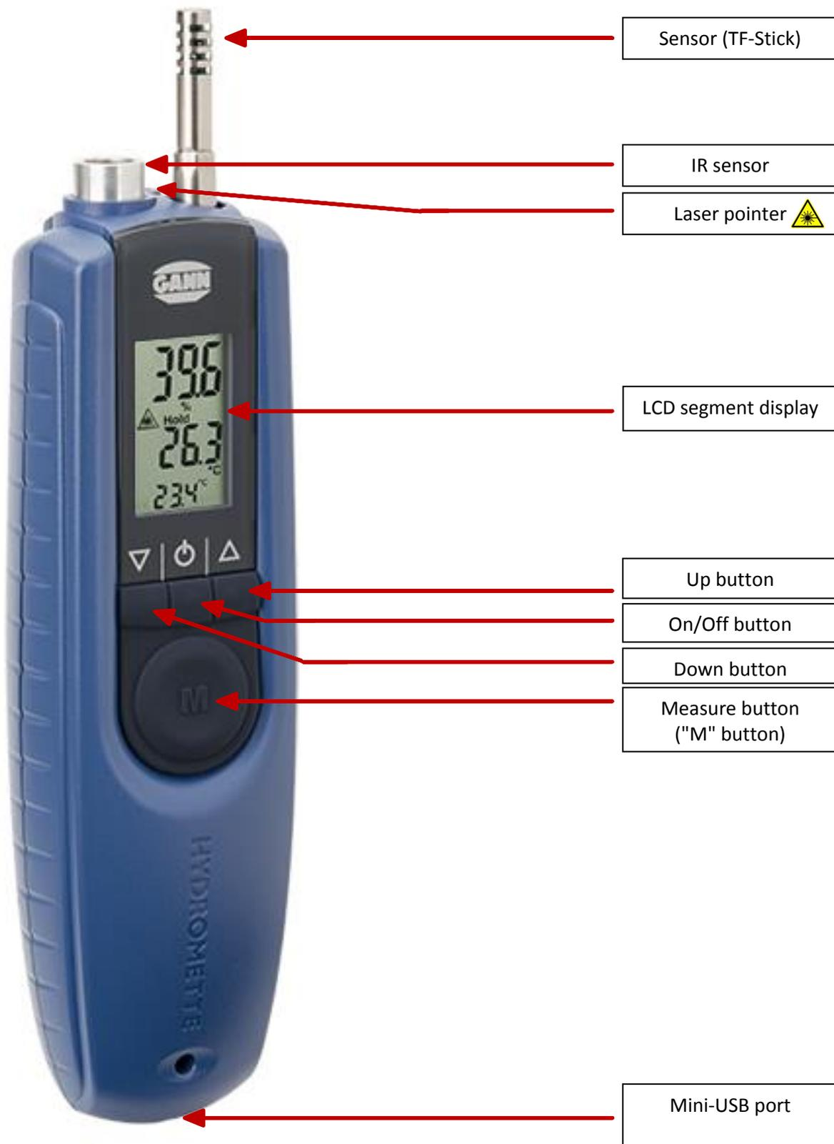
Figure 5-1: Front view of the Hydromette BL Compact TF-IR 2
