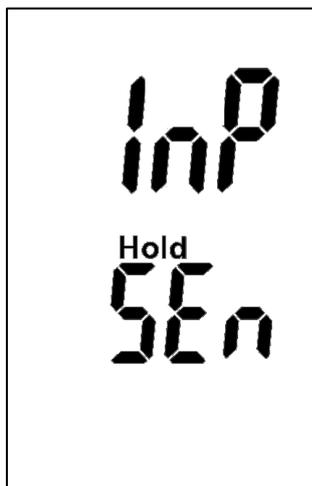
If the TF-stick is not (correctly) inserted, the display "InP SEa" is shown when the measuring button is pressed and held down for a *long time (>2 seconds)*!
