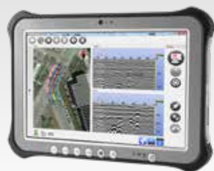
PANASONIC TOUGHBOOK DISPLAYS CARTOGRAPHIC MAP WITH UTILITIES AND GPR PATH
