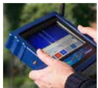
PINPOINT LEAK NOISE LOCALLY ON SITE USING ADVANCED CORRELATION OF ACOUSTIC SIGNALS.
