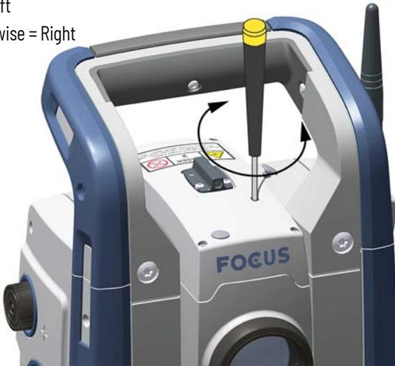
4. Check the alignment of the laser spot and the cross-hairs. Throughout the adjustment procedure, keep the telescope pointing to the adjustment target. The adjusting screws are of a high tension because they are self locking. The screws tighten automatically after you adjust them.
