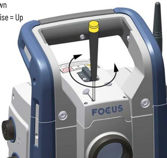
3. To correct the horizontal position of the laser spot, insert the Allen key into the horizontal adjustment port and turn it.
