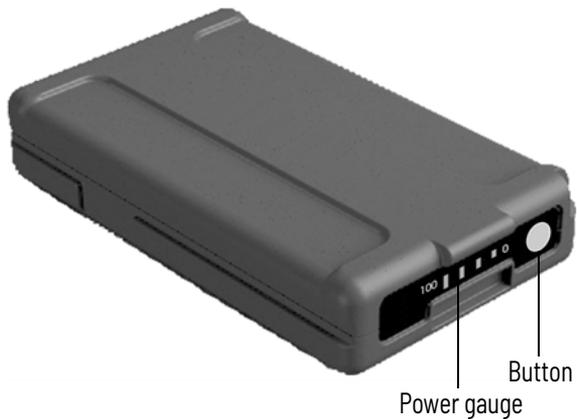
When you press the button, four LEDs on the instrument battery show the power level. Each LED corresponds to a power level of 25% so that when the power level is at 100%, all four LEDs are lit. If the battery is completely discharged, all LEDs are unlit.
