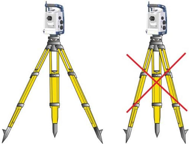
2. Make sure that all the screws on the tripod and/or tribrach are tightened to avoid any play.
