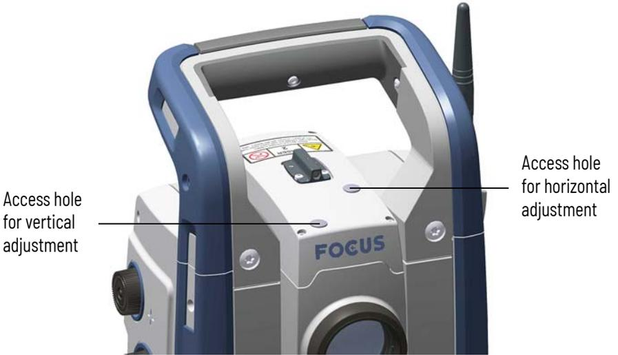
2. To correct the vertical position of the laser spot, insert the Allen key into the access hole for the vertical adjustment screw and turn it.
