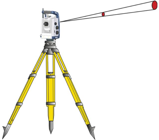
A larger measuring area at longer range is generally better because it enables smaller objects, such as power lines and antennas, to be detected and accurately measured. With a smaller measuring area, these small objects can be easily missed. A smaller measuring area has advantages when measuring tight corners and vertices at close range. When observing measurements to a tight corner, the distance meter beam divergence introduces a range error caused by the size of the sampling area.
