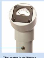
The meter is calibrated 0-100 to indicate a peak response to the Pulse Transmitter signal
