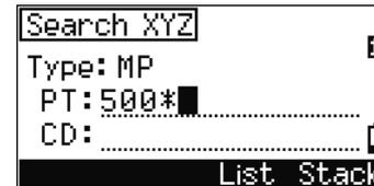
To search by point type, move to the Type field and use **←** or **→** to change the selected point type. The options are ALL, MP, UP, CC, and RE.
