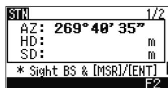
AZ Azimuth calculated by coordinates
