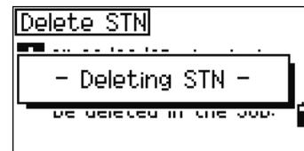
When you delete a ST record in the raw data view or the station data view, all the observation data from the station is also deleted.
