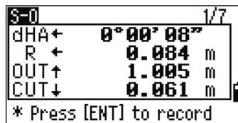
Once a measurement is taken, the Cut/Fill value and Z coordinate are updated as the VA is changed.
