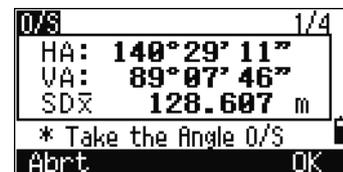
The XYZ data is also recalculated, based on the new angle.
