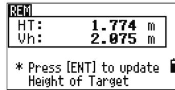
You can use an REM measurement to update the height of target. Take a measurement to the prism, sight the bottom of the prism pole, and press **[ENT]**.
