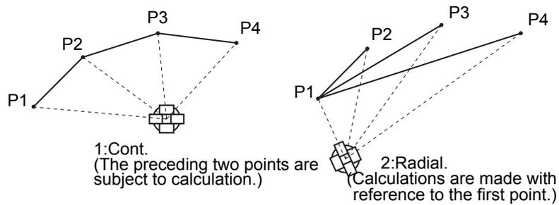
Measuring remote elevation
