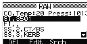
You can edit any field in the ST record, but the instrument does not recalculate any measurements from this station.
