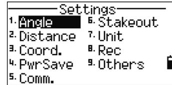
Some job settings, specified in the following sections, cannot be changed once a job is created. If any of these settings are changed while a job is open, a confirmation screen appears, asking you to create a new job with the new settings, or to work with those settings without recording any data. For more information, see [Settings, page 176](#).
