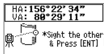
The instrument calculates and records the center of the circle.
