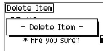
To delete a whole layer, highlight the layer name in the list and press the **DEL** softkey. All codes and layers in the selected layer are deleted.
