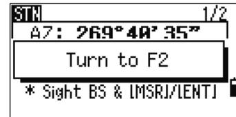
To go directly to the Face-2 measurement after taking a distance measurement to the BS on Face-1, flip the telescope. The instrument automatically detects F1/F2.
