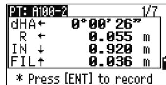
To switch between display screens, press  $\text{[DSP]}$ . This function works as in the angle-distance stakeout, except that the screen counter (for example, S-O1/8) is not displayed. For more information, see [Using \[DSP\] to switch between display screens, page 70](#).
