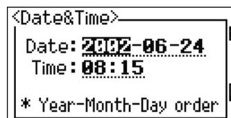
If the highlighted part of the field (for example, the year) is already correct, you can just press **[ENT]** to use the current value. For example, if the date is already set to June 24, 2002, and you want to change the date to June 18, 2002, press
