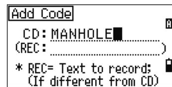
You can use the REC field to define a numeric identifier for each feature code. This is optional: If there is a value in the REC field, this value is stored. If you leave the REC field blank, the CD value is stored.
