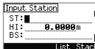
3. Enter the instrument height in the **HI** field and then press **[ENT]**. The cursor moves to the **BS** (backsight point) field.
