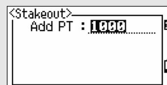
After recording the point, the display returns to the observation screen. When you press  $\text{[ESC]}$ , the display returns to the PT/CD/R input screen. If you entered the stakeout point using a single point name, the PT defaults to the last PT + 1.
