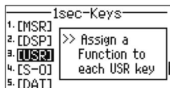
There are two **[USR]** keys. The function that is assigned to each key appears beside the key name.
