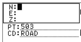
To store the point as an MP record and return to the point input screen, press **[ENT]** in the Z field. The default PT is incremented to the next value.
