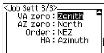
To move between fields, press  $\uparrow$  or  $\downarrow$ . Alternatively, to move to the next field, press  $\text{ENT}$ .
