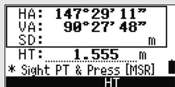
When you have entered three points, the instrument calculates the angle and distances.
