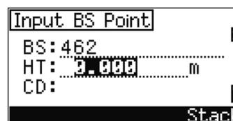
4. Sight the BS on Face-1 (F1). Press  $\boxed{\text{ENT}}$  to complete the setup.
