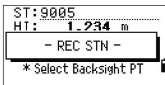
The minimum data required for a resection is either three angle shots, or one angle shot and one distance shot. If you use a distance shot, the distance between the target points must be greater than the measured distance. Stn-Z is calculated from distance-measured data. If no distances are measured, then Stn-Z is calculated using angle-only measurements to points with 3D coordinates.
