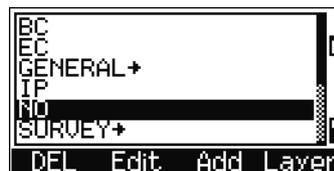
An editing screen appears. For points, the Edit Item screen appears. It contains only the PT field. For codes, the Edit Code screen appears, containing the CD field and the REC field.
