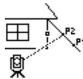
4. Sight the alternative place on the same vertical line as the required target point.
