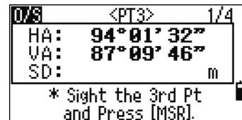
6. If you take a measurement to a fourth point, the corner point can be calculated as the intersection of two walls (P1-P2 and P3-P4). The default elevation is given by P4.
