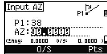
In the Ang field, enter a positive value to rotate the line clockwise. Enter a negative value to rotate the line counterclockwise.
