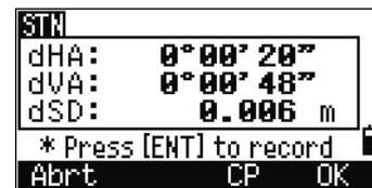
**Sighting the backsight by entering the azimuth angle**
