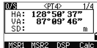
7. Enter a PT (and CD) value. The height of target (HT) defaults to the value used in the last measurement.
