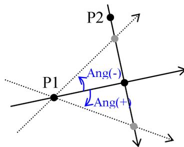
In the O/S field, enter a positive value to specify an offset to the right. Enter a negative value to specify an offset to the left.
