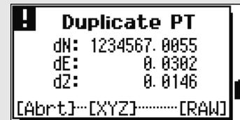
Hold down **[ENT]** for one second to record the measurement as a CP record.
