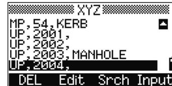
To find a coordinate by name, enter the name in the PT field and press **ENT** twice.
