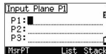
If you press  $\boxed{ENT}$  in a blank field, an input screen for temporary coordinates appears. These coordinates will not be stored.
