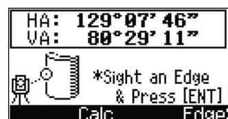
If you have taken a distance measurement to the center of the circle, press the **Calc** softkey to calculate the offset using one edge angle observation.
