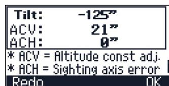
If ACV, ACH, Tilt is out of range, OVER appears. Press any key to return to the first observation screen.
