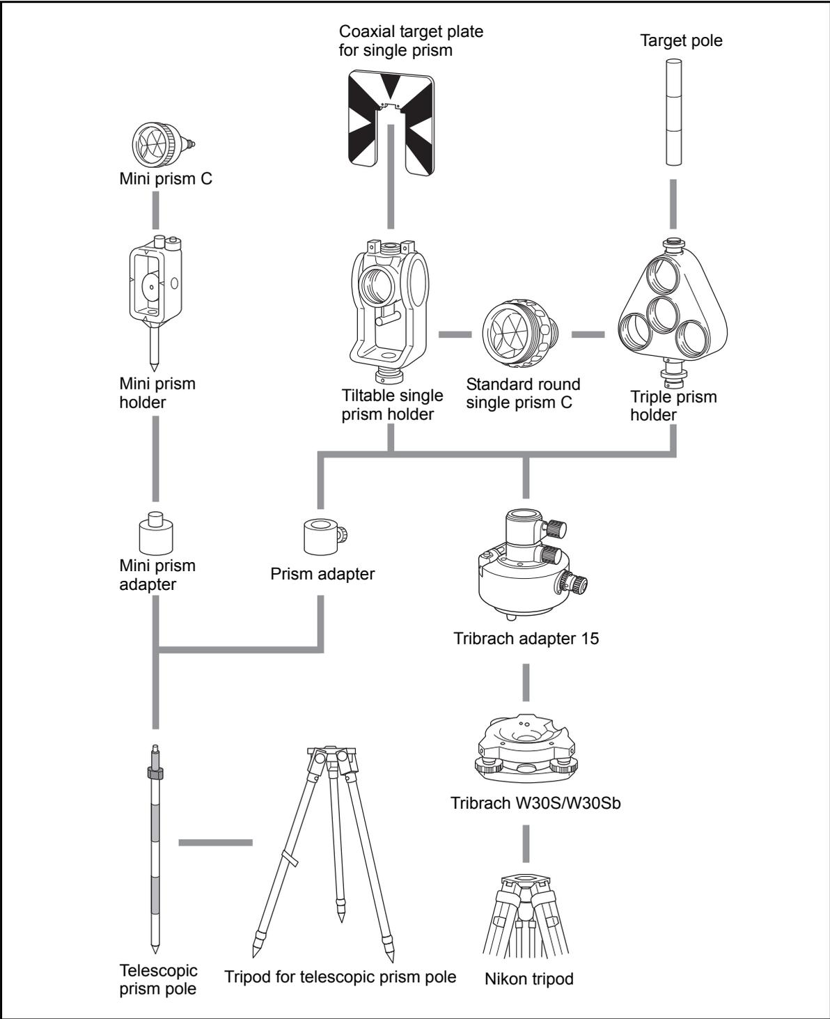
Figure 7.2 Prism reflector side
