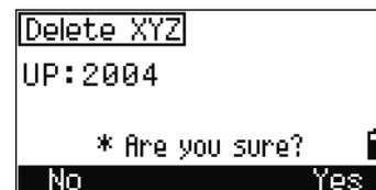
You can also delete coordinate data by pressing the **DEL** softkey in the detailed display screen for the record.
