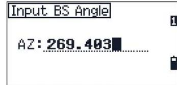
If you press **[ENT]** without entering a value in the AZ field, the azimuth is automatically set to 0°00'00".
