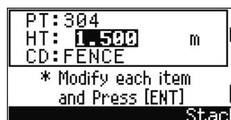
When you change the HT of an SS, SO, or CP measurement record, its Z coordinate is recalculated.
