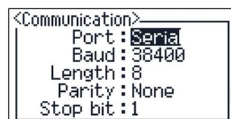
When connecting to a smartphone or tablet via Bluetooth, change port setting to BT Device.
