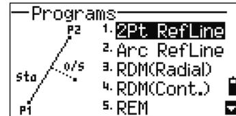
2. Enter the first point for the reference line. Alternatively (to enter the point by measuring), press the **MsrPT** softkey.
