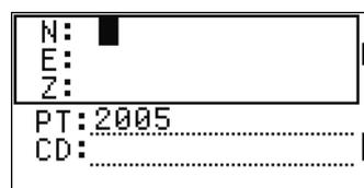
Use the numeric keys to enter the coordinates. Press **ENT** or **v** in each field to move to the next field.
