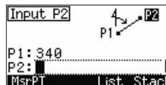
The azimuth, horizontal distance, and vertical distance from the first point to the second point are displayed.
