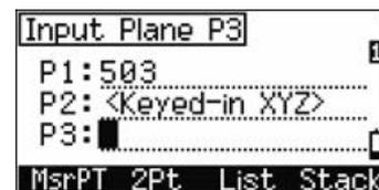
If the plane is defined by two points (by selecting 2Pt), the vertical plane is the same as the plane used in the V-Pln function, but the indicating factors are Sta and dZ, not a and b. For more information, see [Measuring distance and offset values on the vertical plane, page 84](#).
