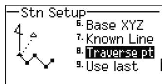
2. Enter a point name or number in the **ST** field and then press **[ENT]**. The cursor moves to the **HI** (height of instrument) field.
