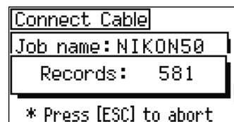
If you press **[ESC]** during data upload, the upload is canceled and the display returns to the Communication menu. Records that were received before you pressed **[ESC]** are stored in the job.
