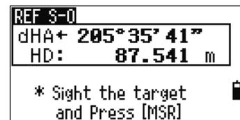
When a distance measurement is taken, the difference from the design point appears.
