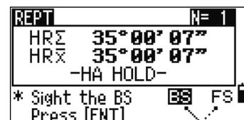
The averaged horizontal angle appears. This value is fixed until the process is finished or cancelled.
