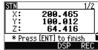
7. To check your measurement, press the **DSP** softkey. If you defined the line by entering its azimuth, HD and VD between P1 and P2 are displayed.
