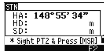
After the measurement to P2 is completed, the coordinates of the station are calculated.
