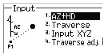
Enter the base point (P1). Type the point name and press **[ENT]**.
