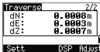
Press the **Sett** soft key to specify the method for distributing the error.
