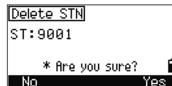
A reconfirmation screen appears. Press the DEL softkey to confirm deletion.
