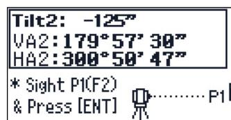
When the observation on F2 is completed, four parameters are displayed.
