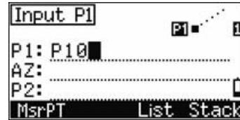
Specify the azimuth bearing. To do this, enter a value in the AZ or P2 field. P2 is a second point on the line.
