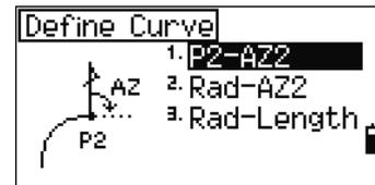
P2 can be any point on the tangent line that is to exit the curve.
