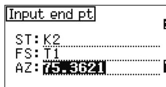
If the end point has no coordinate data, the window on the right will be displayed. Select [Yes] and enter the coordinates of end point. In case of closed-loop traverse, FS also needs to be the known point.
