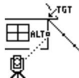
5. To calculate the coordinates and the raw data of the target point, press **[ENT]**.
