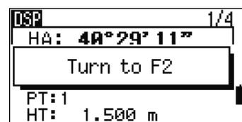
For the HA to be adjusted from a F1/F2 measurement, the Backsight must also have been measured in F1/F2 during the station setup.
