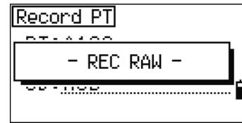
If HA or VA is moved after you take a measurement but before you press **[ENT]**, the angle recorded is the angle shown when **[ENT]** is pressed.
