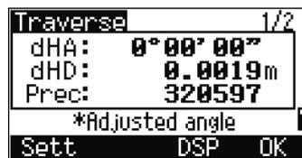
8. Press the  $\square$  soft key or  $\langle \text{ENT} \rangle$ , and the coordinates are calculated allocating the error by the method set for error distribution and recorded.
