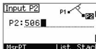
If P1 and P2 are 3D points, the Z coordinate of the perpendicular point is calculated relative to the P1-P2 slope.
