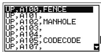
To highlight a point, press **[▲]** or **[▼]**. To go to the stakeout observation screen, press **[ENT]**.
