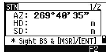
You can also use the **F2** softkey for F1/F2 measurements. See [Advanced feature: Measuring F1 and F2](#), page 58.
