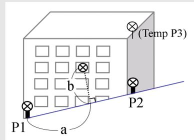
Once the plane is defined, the calculated a and b values are updated as you move the telescope. No distance measurement is required.
