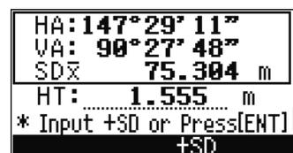
If you use a prism attached to the surface of the circle for the distance measurement, press the **+SD** softkey to eliminate the offset error (from the attached point to the measured surface of the prism) before you press **[ENT]**.
