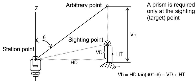
1. To enter the Remote Elevation Measurement function, press **[5]** or select **REM** in the Programs menu.
