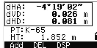
To delete a measurement (because of large sigma values, for example), highlight the measurement data or display the detail screen for the measurement. Then press the **DEL** softkey. The STN coordinates are automatically recalculated.
