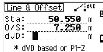
A negative value in the Sta field means the opposite direction along the defined bearing line.
