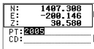
When you press **ENT** in the CD field, the point is stored as an MP record.
