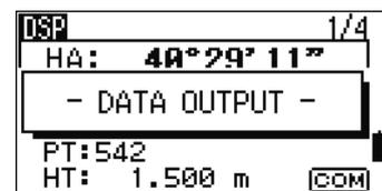
To output data on the COM port when you press **[ENT]**, set the Data Rec field in MENU > Settings > Rec to COM. For more information, see [Recording, page 121](#).
