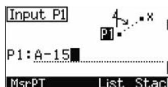
Enter the azimuth, horizontal distance, and vertical distance. Then press **[ENT]**.
