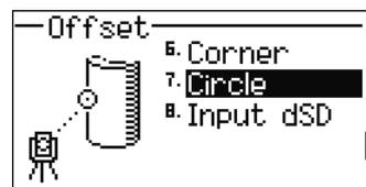
If you have not taken a measurement to the circle before entering this function, a temporary measurement screen appears.
