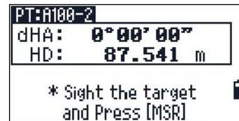
dHA            Difference in horizontal angle to the target point
