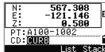
Use the Add Constant field in  $\text{MENU} > \text{Settings} > \text{Stakeout}$  to specify an integer that is added to the point number being staked to generate a new number for recording the staked point. The default value is 1000. For example, when you stake out PT3 with an Add Constant of 1000, the default number for SO record is 1003. For more information, see [Stakeout, page 120](#).
