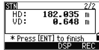
If you defined the line by entering the P2 coordinates, the difference of HD (dHD) and VD (dZ) between your measurement data and input coordinate data are displayed.
