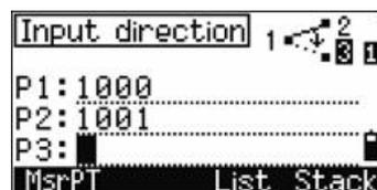
When you press the Msr softkey, a temporary measuring screen appears. Sight the target and press [MSR1] or [MSR2] to take a measurement.
