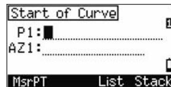
To enter P1 by direct measurement, press the **MsrPT** softkey.
