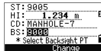
10. To finish the setup and record the station, press **[ENT]** in the BS field.
