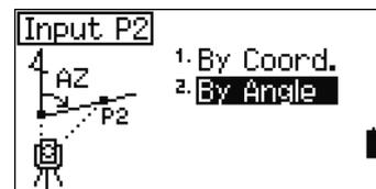
4. If you select **By Angle**, the azimuth input screen appears. Enter the angle value and press **[ENT]**.
