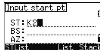
Entering ST displays the Backsight in the BS field and Azimuth in the AZ field.
