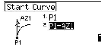
Enter the start of the curve point (P1) and the azimuth of its tangent line (AZ1).
