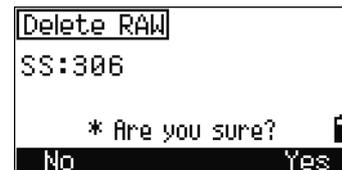
If the Store DB setting is set to Both, the system also deletes the corresponding coordinate data when you delete an SS, SO, or CP record.
