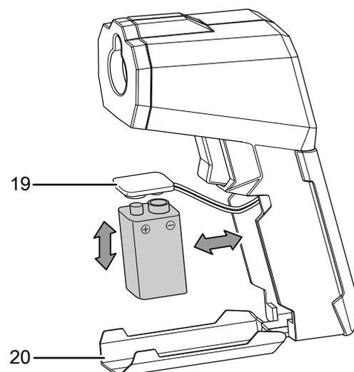
1. Open the battery compartment by folding open the cover (20) with your fingers.
