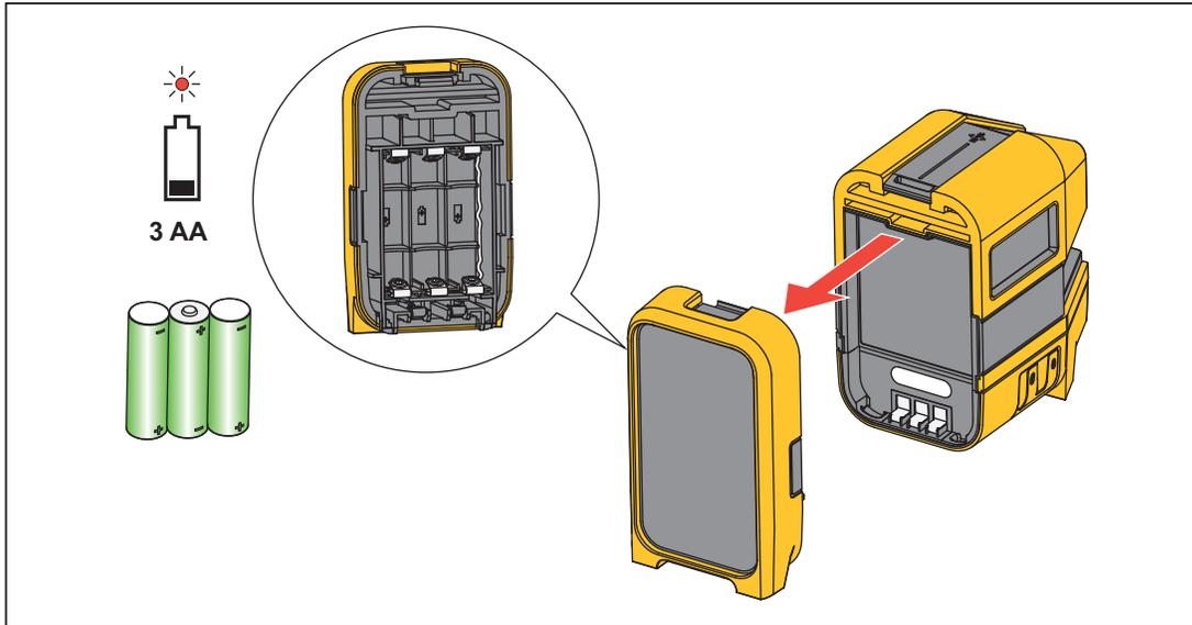
Figure 9. Battery Replacement
