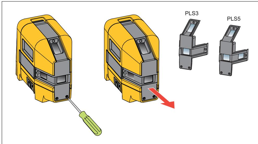
**Figure 10. Housing Glass Insert Replacement**
