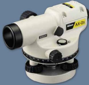
AP/AC/AX Series auto levels are easy to set up and use. All three models can attach to both flat and spherical-head tripods. Horizontal tangent knobs with an unlimited range ensure smooth, precise pointing and angular measurement, and you can operate them with either hand. The detachable eyepiece lens lets you use an optional diagonal eyepiece prism for working in extremely close or steep quarters.
