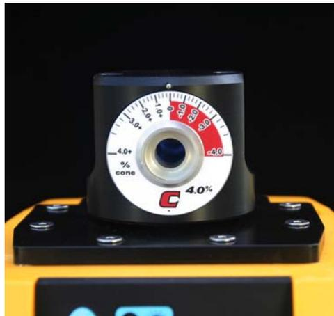
The standard cone scale provide a cone angle of  $\pm 4.0\%$ . There is an optional cone rotor that has a higher resolution scale and provides a cone angle of  $\pm 1.7\%$ .
