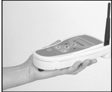
If you connect the radio remote control to a grade rod, and the radio remote control is oriented vertically, the antenna should point upward from the top of the radio remote control.
