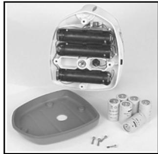
3. Put the battery-housing compartment in place and reinstall the four screws.
