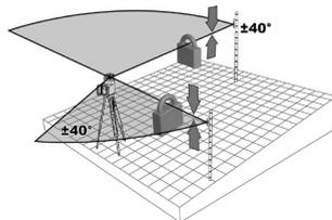
**Note:** In every PlaneLok mode the laser continues to servo to the receiver's signals. Any loss of signal over an extended period of time (1 minute) causes the laser to go into the HI-alert condition (beam turns off, rotor stops and a warning message occurs at the LCD. PlaneLok mode can be reactivated after the error message has been deleted with button 4. Exiting of PlaneLok mode can be done by pressing button 3 (ESC) or any HL760 button.
