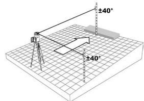
1. Set up the laser over the reference point.
