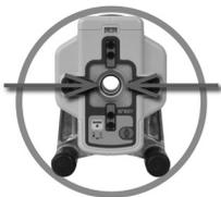
**Automatic-Spot Alignment:** SF601 guides the beam to the target point in the horizontal axis, while the Z-axis grade value will be maintained.
