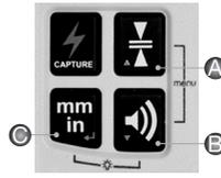
Next, turn on the receiver then press and hold the Deadband (A) and the Audio (B) buttons for two seconds. After two seconds the display shows MENU first, then RDIO.
