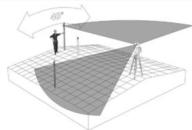
1. Set up the laser over the reference point.
