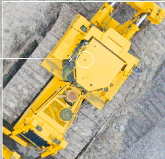
WingtraOne can map this quarry in an hour's flight. The resolution of the final map allows you to zoom in and see this very coin lying on the ground. And what is best – it is possible to know the exact coordinates of the coin down to an absolute accuracy of 1 cm (0.4 in).
