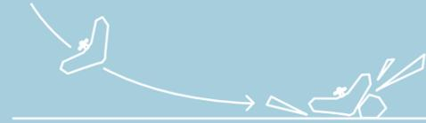
Drone deteriorates with each landing and risks to be broken on rocky terrain
