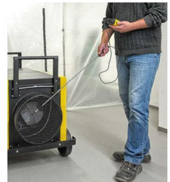
*The slim telescopic probe of the TA300 can be variably extended to an effective length of 1 m, thus measuring applications can be carried out with more ease. Also convenient for flow rate measurements in remote or poorly accessible locations or inside air ducts and ventilation shafts.*
