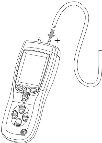
2. Press the P/V/F button (11) until *PRESS* appears in the measuring mode display (35).
