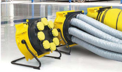
Up to eight 100 mm hoses can be attached to the combination distributor and in case of high central capacity requirements also a 450 mm air hose. For ventilation over longer distances we recommend the combined application with the 250 Pa high-pressure fan TTV 4500 HP.
