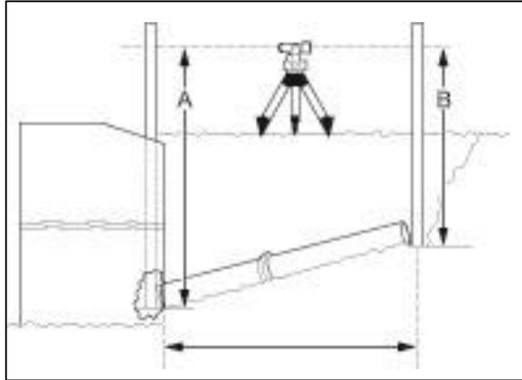
After the first 25 – 50 feet (8 – 15 m) of pipe has been laid, it is recommended that you make a grade check to insure that the setup is correct, and that the system is properly operating.
