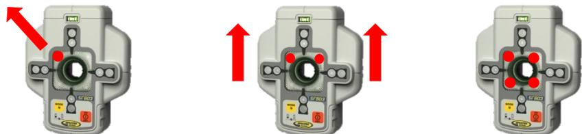
**Line Scan** - For a faster second day setup, line scan enables complete automatically movement of the laser beam to the left and right limits. Press and release the **M** button at the standard display and select **Line Scan** using the **(+)/(-)** and **left/right** buttons.
