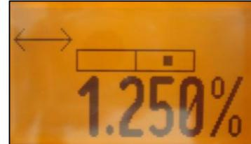
Corrections for centering the beam at the target can be done using the **left/right** buttons.
