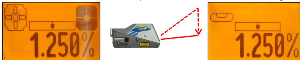
Automatic Spot Align can be exited any time by pressing and releasing **ESC** button.
