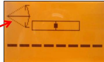
Using the **+** or **-** button at the RC803 remote control or at the laser stops the automatic upwards beam movement. Adjust the beam using **Left/Right** buttons until the beam is centered at the line stake. After aligning the beam to the required direction position, pressing and releasing the **E** button starts the beam plumb down movement to the previous dialed in grade value.
