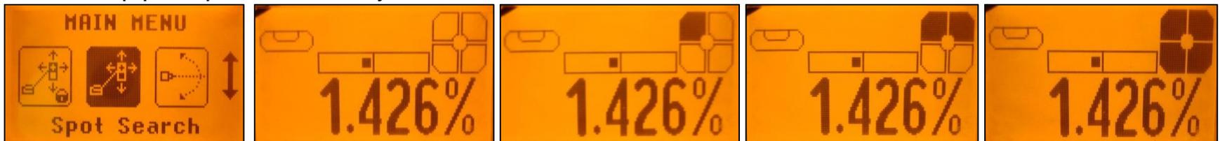
Manual Spot Search can be exited any time by pressing and releasing **ESC** button.
