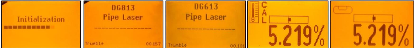
**Don't start automatic functions at the menu before the reference check has been finished.**
