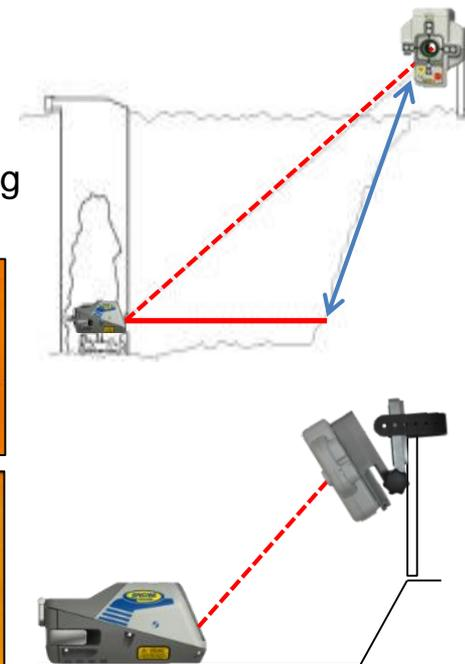
**Automatic Spot Match (only DG813)** - Automatic-Spot-Match can be used for measuring an unknown grade value in an existing pipe or open trench.
