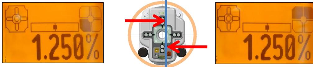
When the alignment is finished, the beam moves plumb down to the dialed in grade value.
