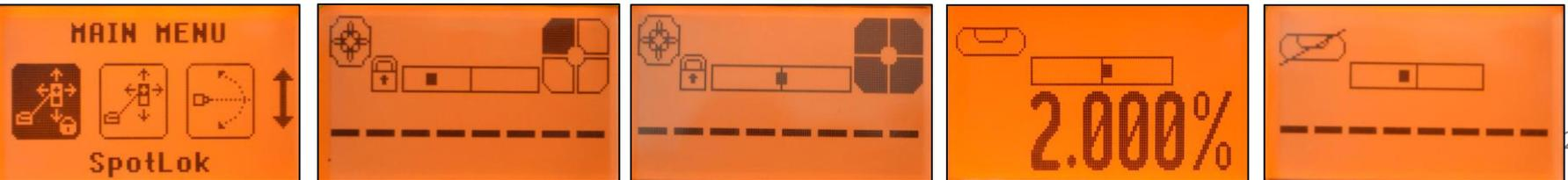
**Manual Spot Search Mode (only DG813)** - The Spot Search mode is used for pipe laying by detecting the beam manually using the **Spot Finder SF803** and can be activated in **automatic and manual mode**.
