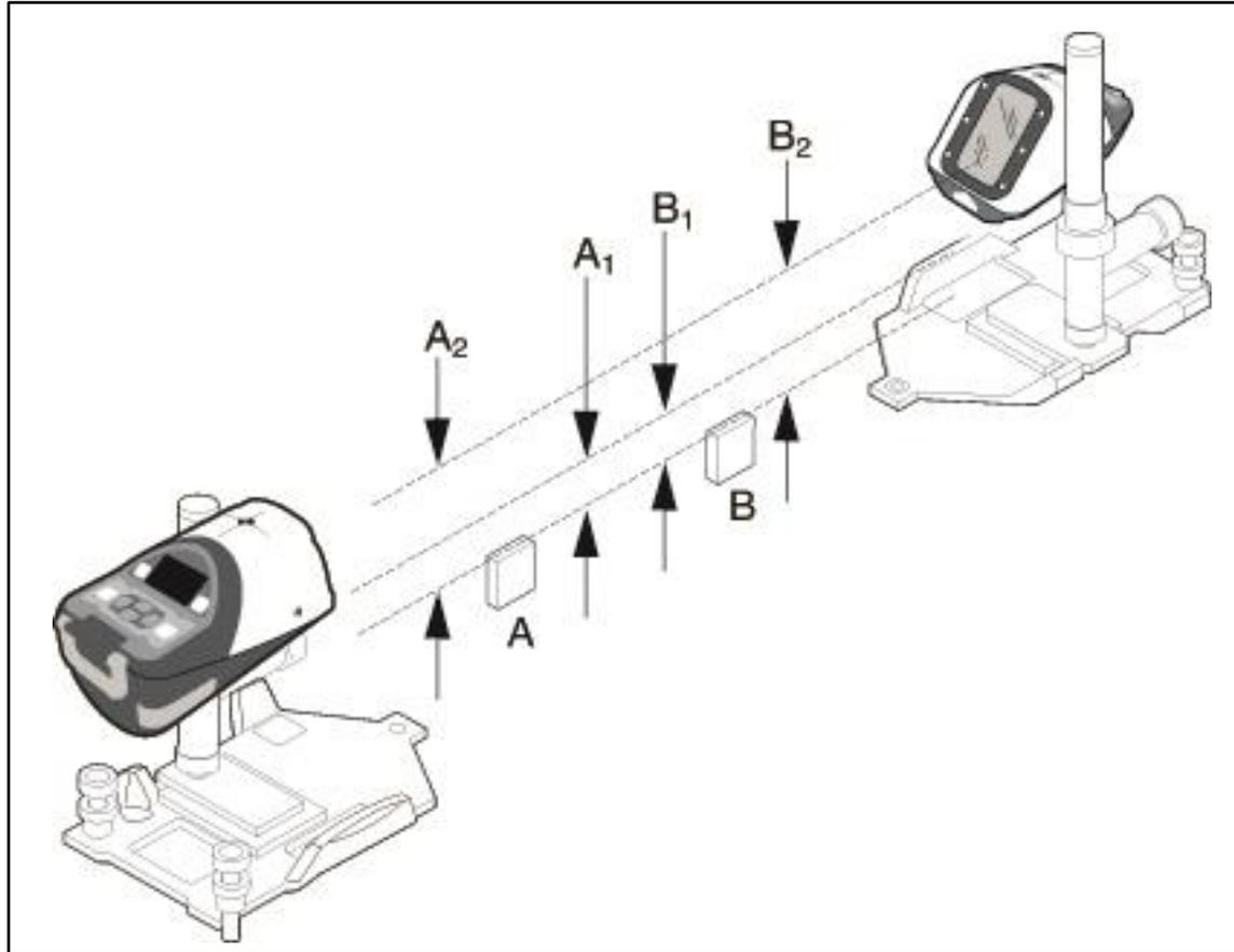
Checking the calibration of your pipe laser is easy. All you need is an engineer's rule and your pipe laser.
