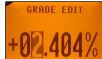
Grade Entering can be exited any time by pressing and releasing **M** button.
