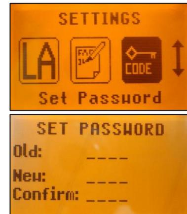
Press and release **E** button to **store the selected password**; unit falls back to the standard display.
