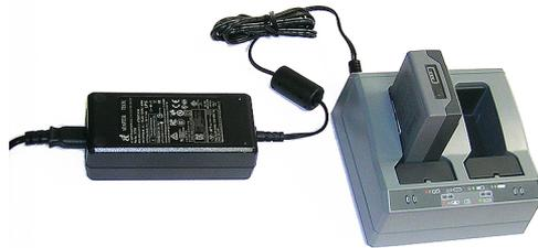
Charging takes approximately 3 hours at room temperature. If two batteries are inserted in the battery charger, then the batteries will be charged sequentially, from left to right.
