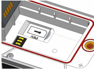
To extract the SIM card, gently push it a bit further in. This releases it from the slot. Just let go before extracting the SIM card from the battery compartment.
