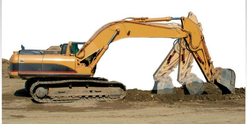
ACE AUTOMATICALLY CALCULATES AND CORRECTS THE GRADE DISPLAY FOR THE ANGLE OF THE DIPPER ARM. THE 'ON GRADE' LEVEL CHANGES AS THE ARM IS EXTENDED OR RETRACTED UP TO 30 DEGREES.
