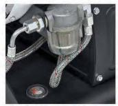
The filling level of the integrated fuel tank can be checked anytime via the standard liquid level indication.
